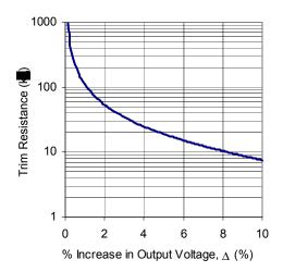
The value of Vref can be found in the Electrical Data section of this data sheet. The maximum power available from the power module is fixed. As the output voltage is trimmed up, the maximum output current must be decreased to maintain the maximum rated power of the module. It is also desirable to slightly increase the input voltage while trimming up the output with heavy load current.
